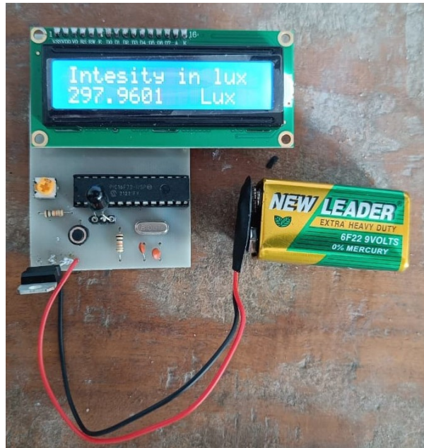
Figure 5.2: Final PCB board Implementation
